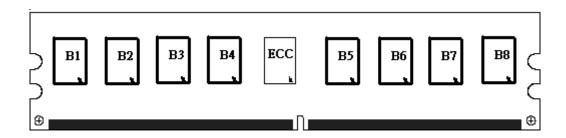
2. Following by two steps of ECC U-DIMM test are applied on the dies of module. First step, to use JET-5451/JET-5452 DDRII/DDR III Extender to make the normal 64 bit ECC U DIMM test for those dies of module. With turning off ECC on module to make sure all dies are working normally.
