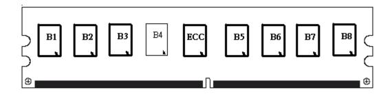
3. The further test is to use JET-5450 DDRII 240 ECC Extender/JET-5455 DDRIII 240 ECC Extender/to active ECC and turn off B4 die for the next test to make sure ECC is in normal function.
